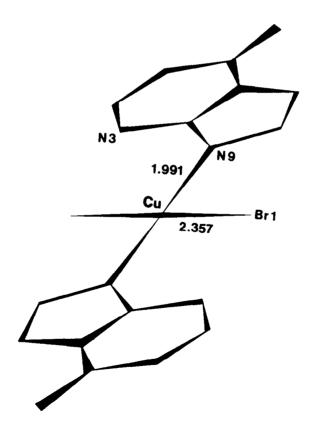
A schematic view of the [Cu(adeH)<sub>2</sub> Br<sub>2</sub>]<sup>2+</sup> ion looking down the diad axis through the copper atom. Standard deviations are Cu\_Br, 0.003; Cu\_N, 0.010A.
